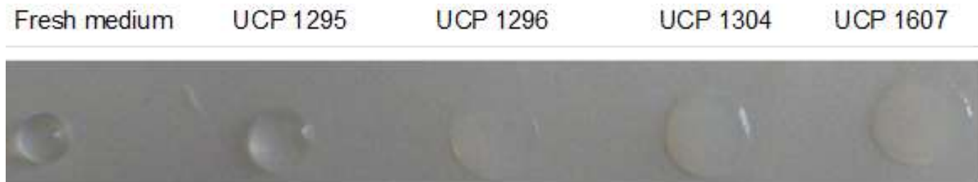
Figure 2. Tensioactivity of crude biosurfactants of the Rhizopus strains on parafilm M hydrophobic surface.
